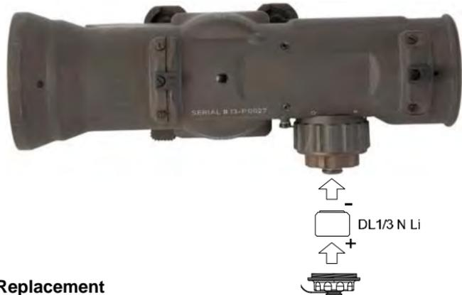
**Figure 4-1: Battery Replacement**
