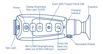
Power Button - The Scout II has three power states: On, Off, and Auto Shutdown.
